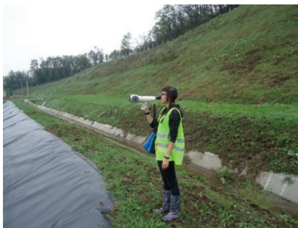
Figure 1. Field odour measurement by field olfactometer – Nasal Ranger (Kopányi, 2014)
